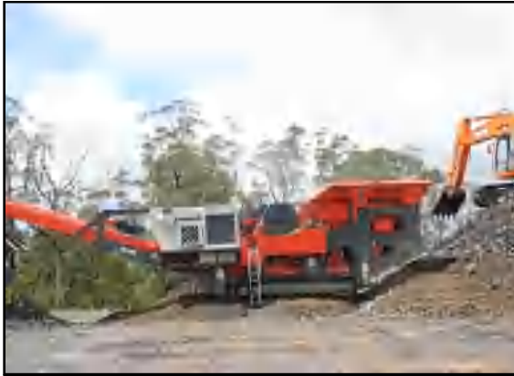
PHOTOGRAPH 3: Crusher working in quarry pit at Sheridan's Hard Rock Quarry
